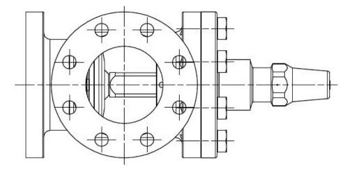
The valves come with two flange connections.
